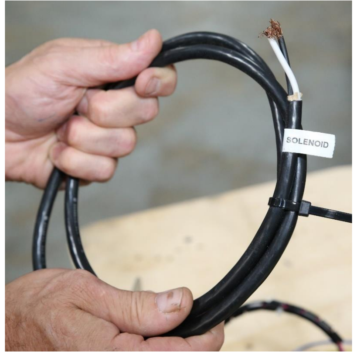
The Solenoid Cable is wrapped up and labeled. This is for a 208/240VAC Solenoid Valve Coil.
