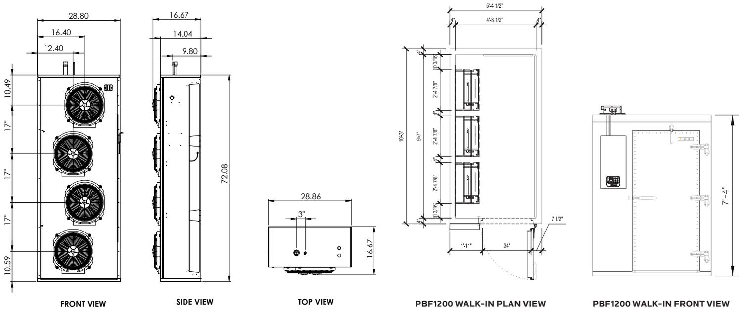
PBF1200-TS includes three evaporator coils
